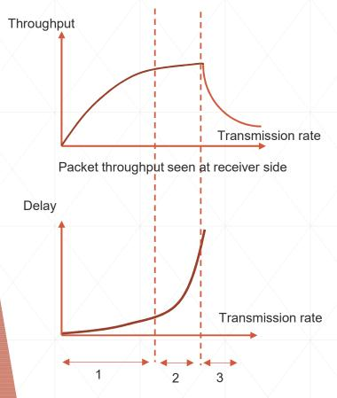
Packet delay seen at receiver side
