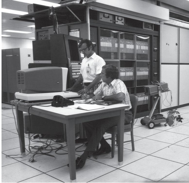
**FIGURE 7.14.1 The Illiac IV control unit followed by its 64 processing elements.** It was perhaps the most infamous of supercomputers. The project started in 1965 and ran its first real application in 1976. The 64 processors used a 13-MHz clock, and their combined main memory size was 1 MB:  $64 \times 16$  KB. The Illiac IV was the first machine to teach us that software for parallel machines dominates hardware issues. Photo courtesy of NASA Ames Research Center.
