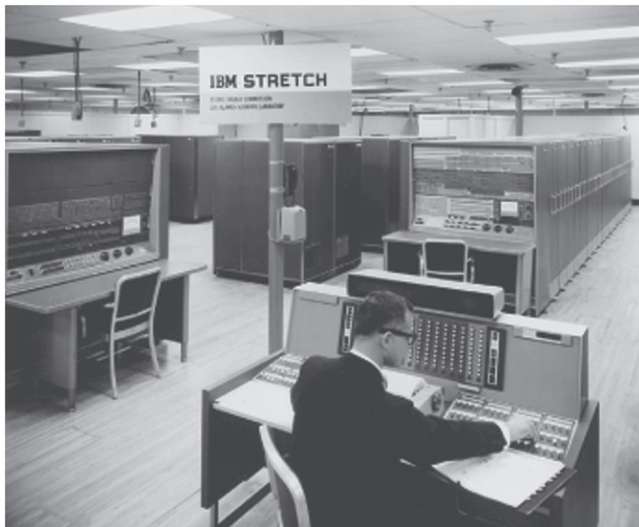
**FIGURE 4.15.1** The Stretch computer, one of the first pipelined computers.
