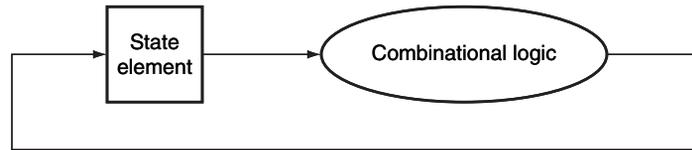
**FIGURE C.7.3** An edge-triggered methodology allows a state element to be read and written in the same clock cycle without creating a race that could lead to undetermined data values. Of course, the clock cycle must still be long enough so that the input values are stable when the active clock edge occurs.
