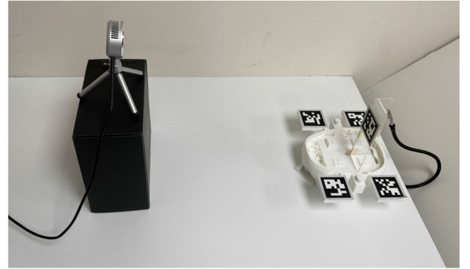
FIGURE 4 Experimental setup used for data collection. Note the fixed placement of the camera and skull. Also note the use of the laser cut wedged and magnetic arm that was used to hold setup still for data collection
