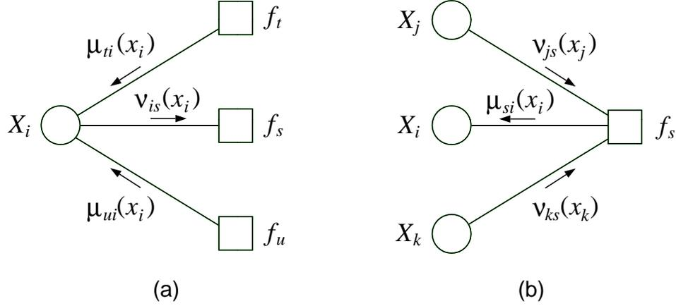
Figure 4.10: (a) The computation of the message  $\nu_{is}(x_i)$  that flows from factor node  $s$  to variable node  $i$ . (b) The computation of the message  $\mu_{si}(x_i)$  that flows from variable node  $i$  to factor node  $s$ .
