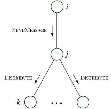
Figure 4.5: A sequential implementation of the SUM-PRODUCT algorithm for a tree  $\mathcal{T}(\mathcal{V}, \mathcal{E})$ . The algorithm works for any choice of root node, and thus we have left CHOOSE-ROOT unspecified. A call to COLLECT causes messages to flow inward from the leaves to the root. A subsequent call to DISTRIBUTE causes messages to flow outward from the root to the leaves. After these calls have returned, the singleton marginals can be computed locally at each node.
