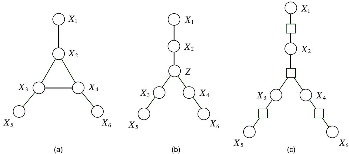
Figure 4.14: (a) An undirected graphical model in which the center cluster of nodes is assumed to be parameterized as a non-factorized potential,  $\psi(x_2, x_3, x_4)$ . (b) An equivalent undirected model based on the “super-variable”  $Z$ . (c) An equivalent factor graph.
