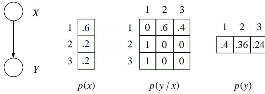
Figure 4.16: The marginal and conditional probabilities for a pair of variables  $(X, Y)$ . The maximizing values of the individual marginals are  $X = 1$  and  $Y = 1$ , but the configuration  $(X = 1, Y = 1)$  has zero probability.
