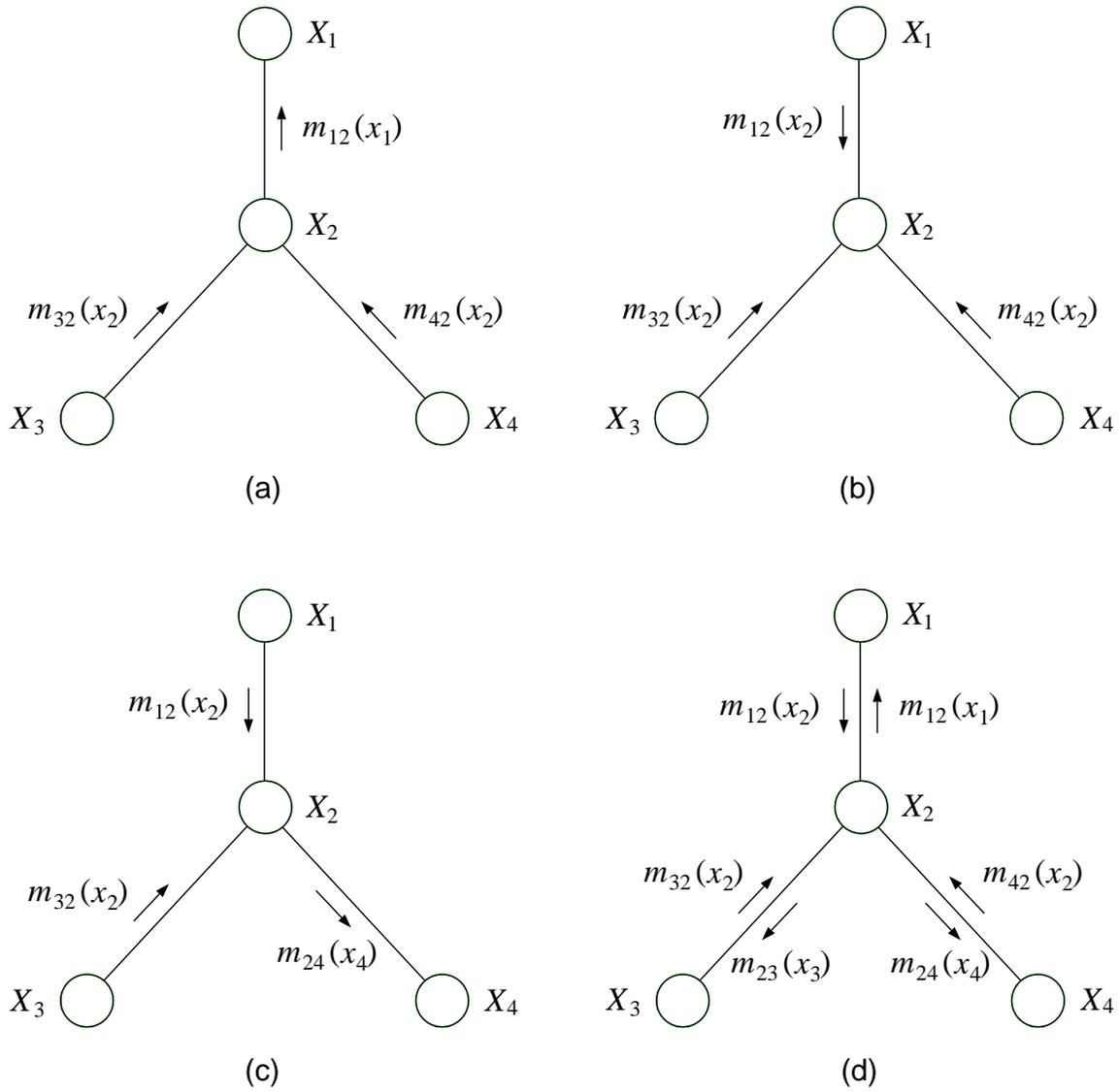
Figure 4.3: (a) The messages formed when computing the marginal of  $X_1$ . (b) The messages formed when computing the marginal of  $X_2$ . (c) The messages formed when computing the marginal of  $X_4$ . (d) All of the messages needed to compute all singleton marginals.
