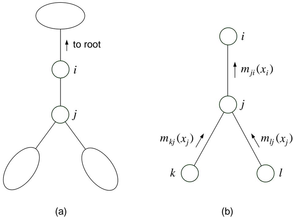
Figure 4.2: (a) A fragment of an undirected graph. Nodes  $i$  and  $j$  are neighbors, with  $i$  nearer to the root than  $j$ . (b) The messages that are created when nodes  $k$ ,  $l$  and  $j$  are eliminated.
