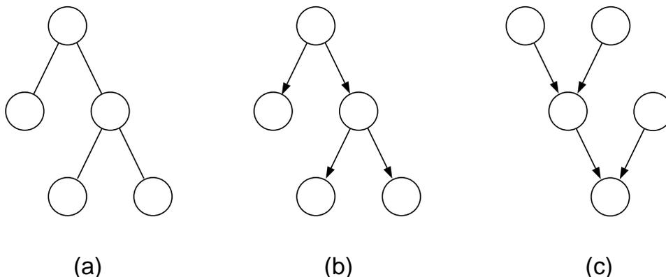
Figure 4.1: (a) An undirected tree. (b) A directed tree. (c) A polytree.
