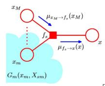
$$\mu_{f_s \to x}(x) = \sum_{x_1} \dots \sum_{x_M} f_s(x, x_1, \dots, x_M) \prod_{m \in \text{ne}(f_s) \setminus x} \left[ \sum_{X_{sm}} G_m(x_m, X_{sm}) \right]$$
