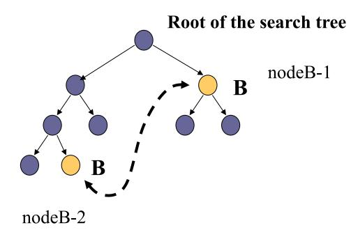
**Case B**: nodes with the same state are not on the same path from the initial state
