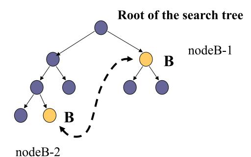
**Conclusion: Since we are happy with the optimal solution nodeB-2 can be safely eliminated.** It does not affect the optimality of the solution.
