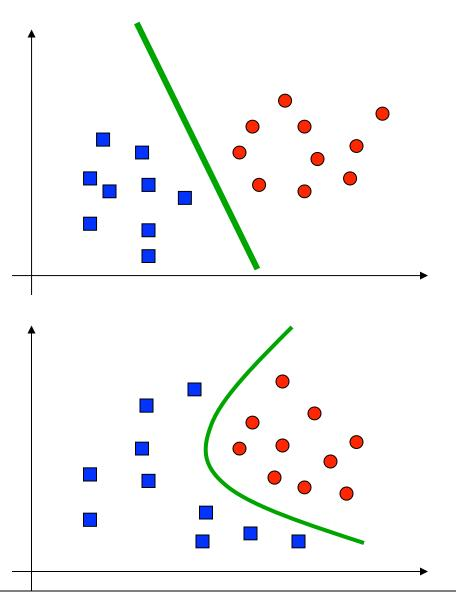
Linear separator in the expanded feature space
