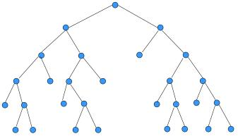
**Backpruning:** Prune branches of the tree built in the first phase in the botton-up fashion by using the validation set to test for the overfit
