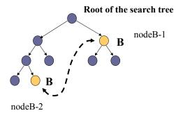
Since we are happy with the optimal solution nodeB-2 can be eliminated. It does not affect the optimality of the solution.
