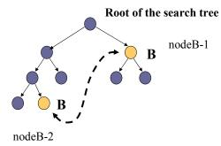
**Case B**: nodes with the same state are not on the same path from the initial state
