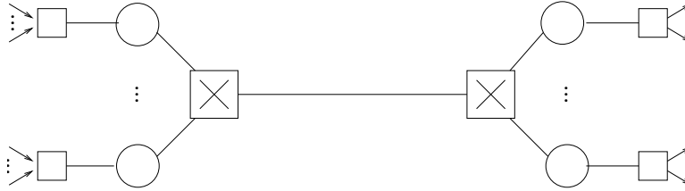
Figure 7. Single-bottleneck topology with n forward and n reverse trunks
