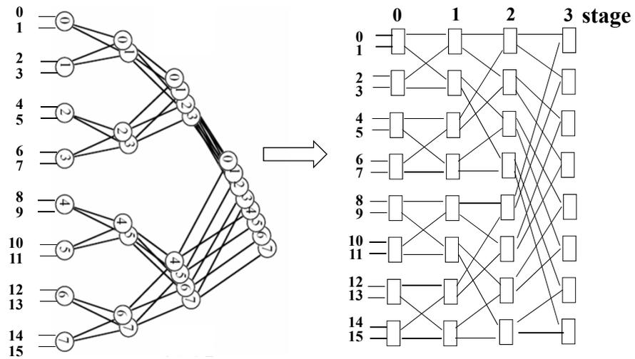
A fat tree networks using 2x2 bidirectional switches
