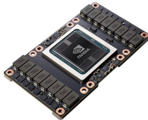
NVIDIA Tesla V100 = 125 TFLOPs of compute
