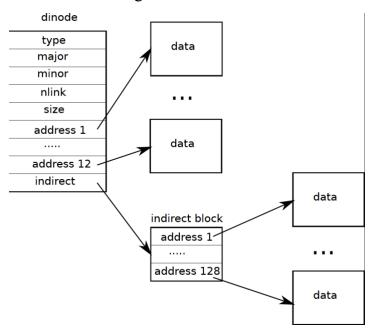
The code that finds a file's data on disk is in <code>bmap()</code> in <code>fs.c.</code> Have a look at it and make sure you understand what it's doing. <code>bmap()</code> is called both when reading and writing a file. When writing, <code>bmap()</code> allocates new blocks as needed to hold file content, as well as allocating an indirect block if needed to hold block addresses.
