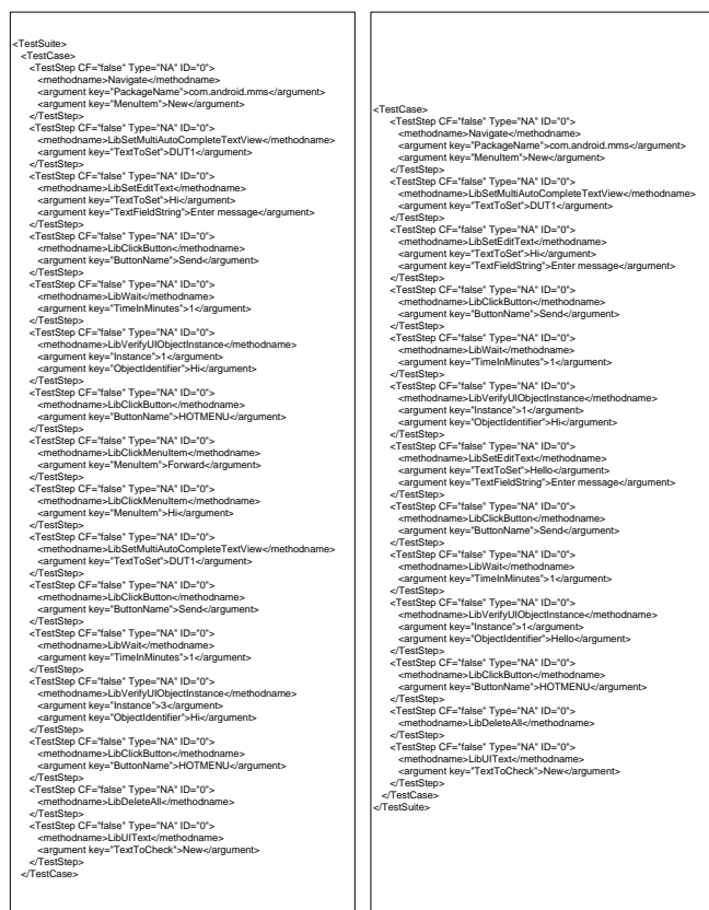
Fig. 29. XML generated for Forward-Reply test cases
