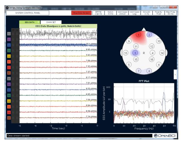
The version of our OpenBCI boards support 16 channels data recording. That is, the system can monitor EEG signal from different 16 position on the head at the same time. It provides us more data for further analysis, especially in machine learning process, more data always represent a better prediction model. The following picture shows the 16 channels and corresponding position on the head, respectively.
