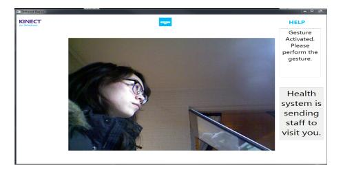
The Help label is grey tag after system initialization. When the system recognizes that a user speaks "HELP", the tag will change into blue. And then the gesture recognition is activated, which means the user could perform the gesture at this moment. Once the system recognizes the gesture, it will send an alert message to the
