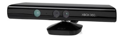
Kinect for Xbox 360, or simply Kinect, is a motion sensing input device by Microsoft for the Xbox 360 video game console. Based upon a webcamstyle add-on peripheral for the Xbox 360 console, it enables users to control and interact with the Xbox 360 without the need to touch a game controller, through a natural user interface using gestures and spoken commands.
