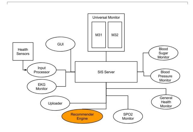
**Illustration 0: SIS component network with Recommender Engine**
