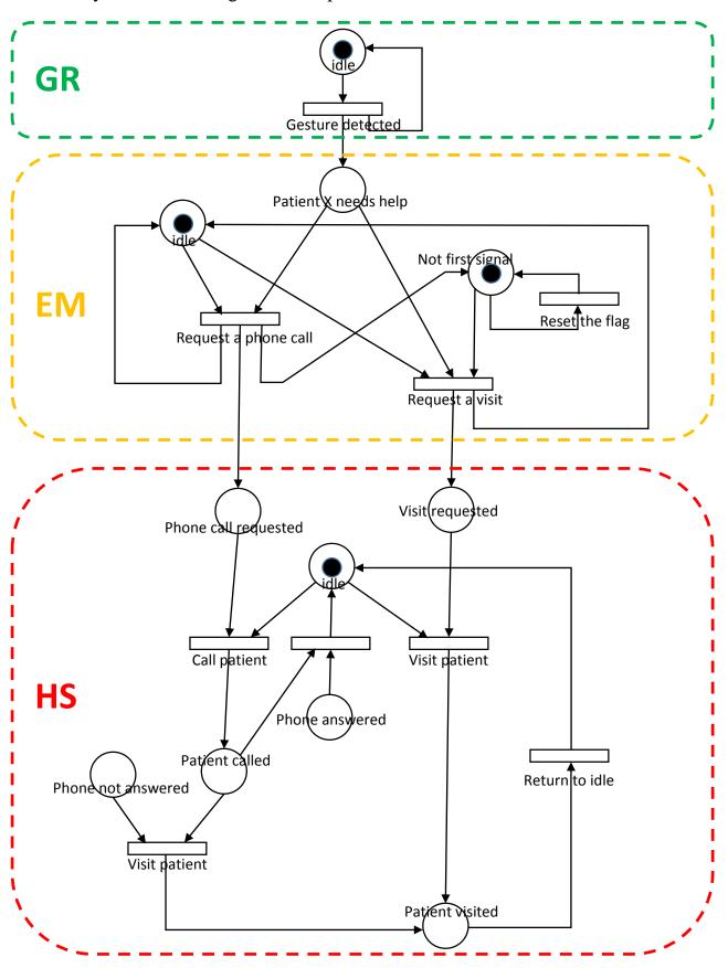
(c) Suppose the emergency manager index cell corresponds to a **super-component**, i.e., the emergency manager can enumerate a number of feasible solutions and select the most appropriate one. Draw the personal health care system as a pair of (I-card, C-card), and convert it into an ordinary Petri net. (To do that, you need to assume a specific number of feasible solutions for the emergency manager to evaluate. Let us say three.)
