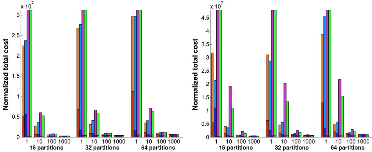
Figure 4. Normalized total cost (communication volume + (migration volume)/ $\alpha$ ) for auto dataset with (a) perturbed data structures and (b) perturbed weights. Each group of four bars represents results for Zoltan-repart, ParMETIS-repart, Zoltan-scratch and ParMETIS-scratch, from left to right respectively.
