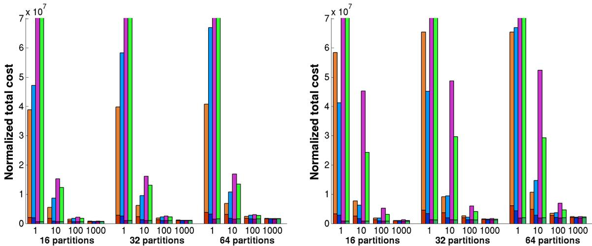
Figure 5. Normalized total cost (communication volume + (migration volume)/ $\alpha$ ) for apoa1-10 with (a) perturbed data structures and (b) perturbed weights. Each group of four bars represents results for Zoltan-repart, ParMETIS-repart, Zoltan-scratch and ParMETIS-scratch, from left to right respectively.
