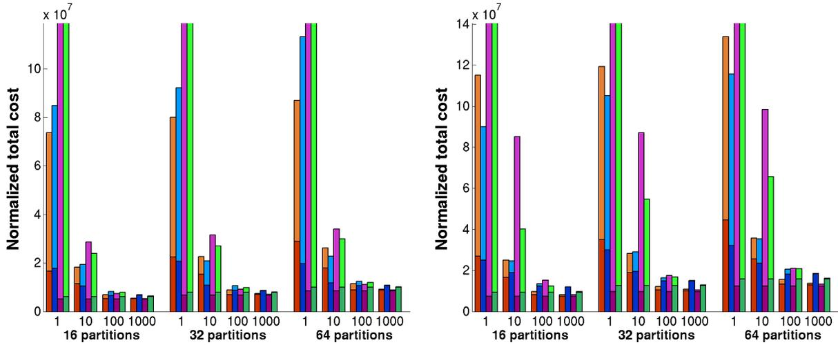
Figure 6. Normalized total cost (communication volume + (migration volume)/ $\alpha$ ) for cage14 with (a) perturbed data structures and (b) perturbed weights. Each group of four bars represents results for Zoltan-repart, ParMETIS-repart, Zoltan-scratch and ParMETIS-scratch, from left to right respectively.
