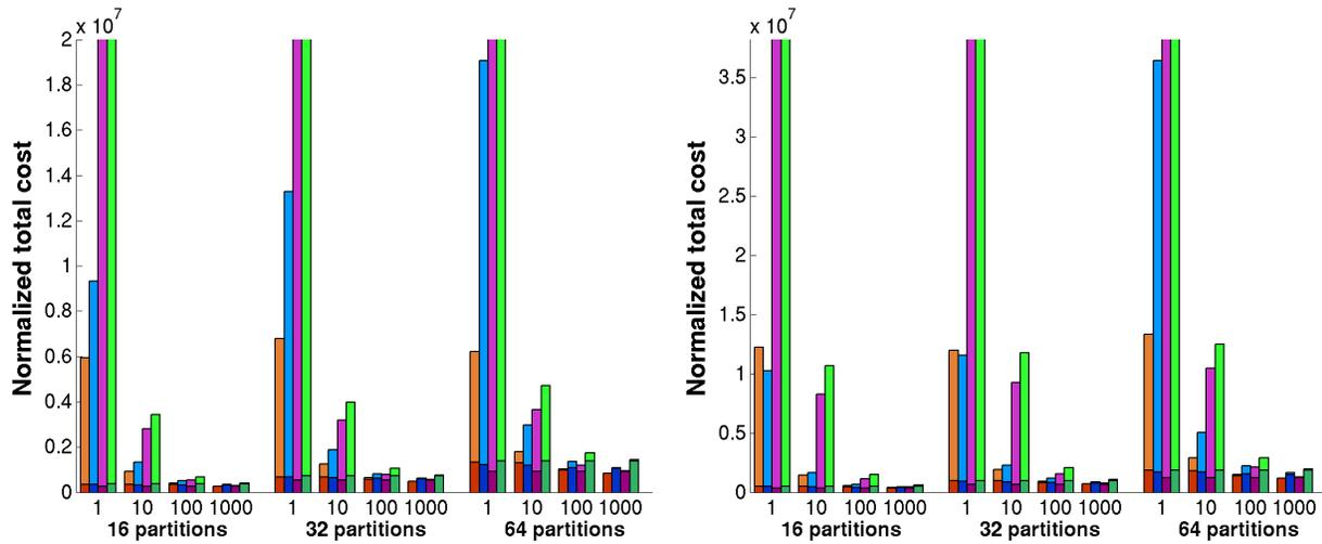
Figure 3. Normalized total cost (communication volume + (migration volume)/ $\alpha$ ) for 2DLipid with (a) perturbed data structures and (b) perturbed weights. Each group of four bars represents results for Zoltan-repart, ParMETIS-repart, Zoltan-scratch and ParMETIS-scratch, from left to right respectively.
