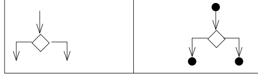
Figure 9: Diagrammatic and graph representation of a decision unit
