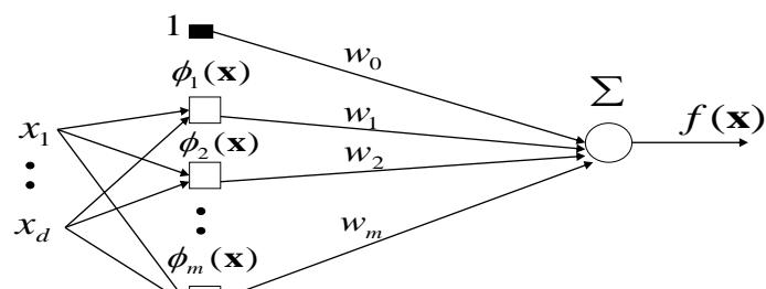
Original input  $\rightarrow$  New input  $\rightarrow$  Linear model
