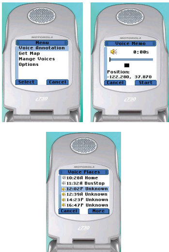
figure 4. Cell phone interfaces for Voice. 4.1 Initial interface after activation. 4.2 voice capture interface, 4.3 voice history. After pressing the ok button in 4.3, the DText interface will pop up.
