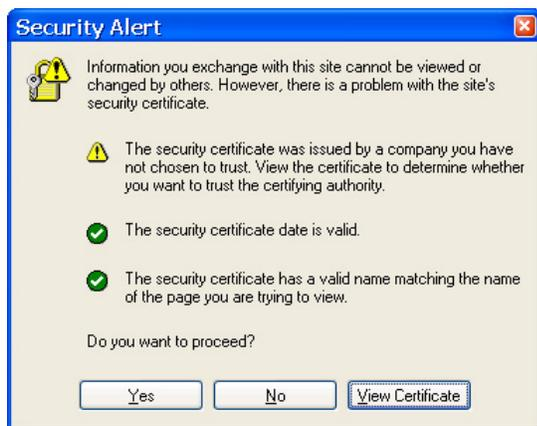
**Figure 2: Internet Explorer 6.0 dialog when server certificate cannot be verified because public key of issuing CA is unknown.**
