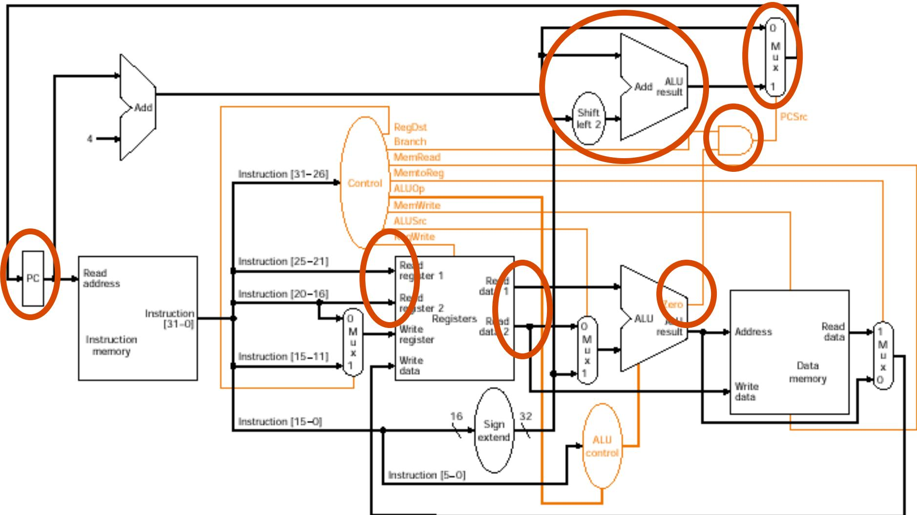
*Read and compare sources, generate zero & branch control, compute target address, update PC if zero and branch*
