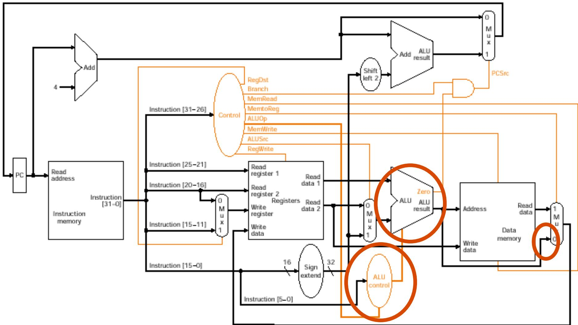
*ALU operates on data from register file, ALU control determined* 79
