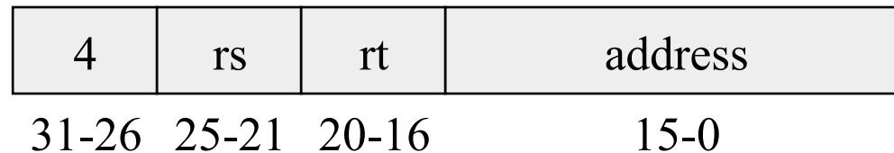
*Destination register in one of two places: 15-11 for arithmetic and 20-16 for load; need multiplexor on write register address*
