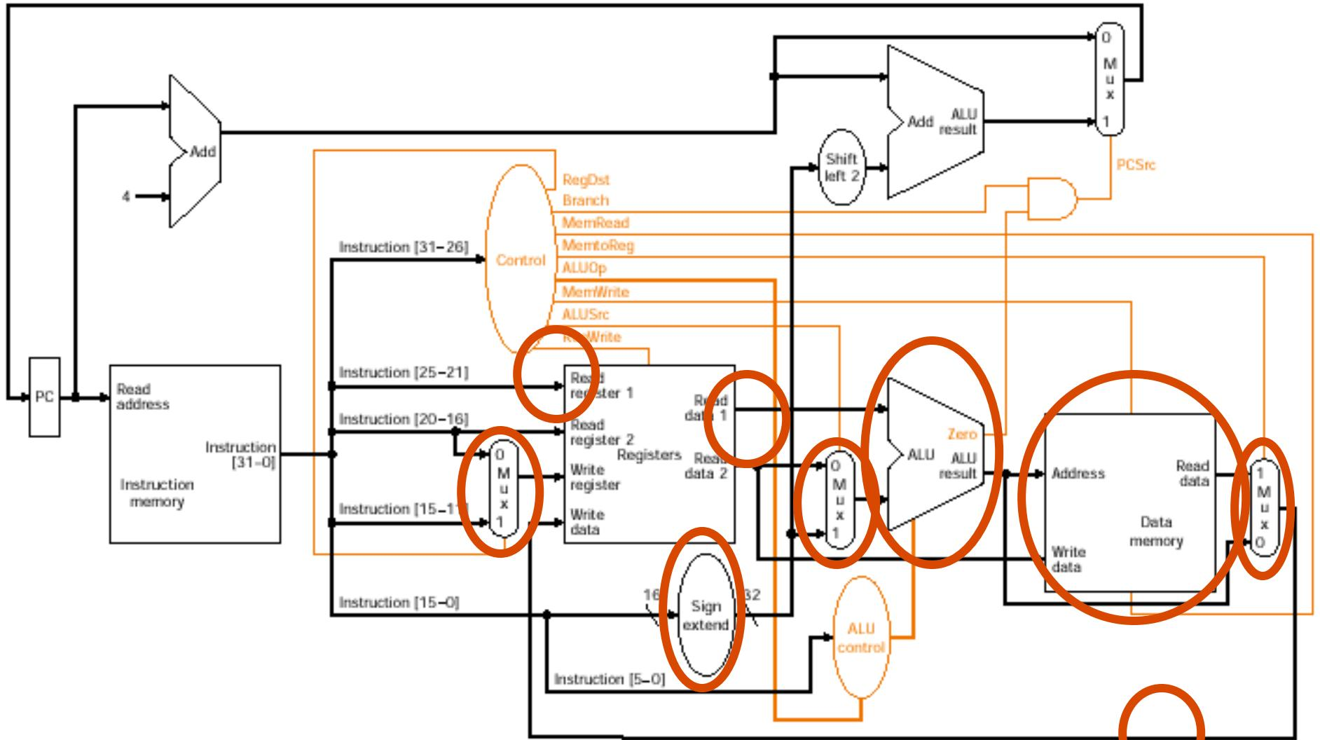
*Only one source reg to read, sign extend, form address, write to destination in different position in instruction (bits 20-16)*
